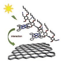
**Exfoliation of graphite** was achieved using a zinc phthalocyanine oligomer that is also an electron donor. The resulting functionalized graphene material was investigated by Raman and electron spectroscopy and was trialed in a photoelectrochemical cell.
