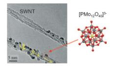
Charging clusters: A hybrid of polyoxometalate (POM) molecules individually adsorbed onto the surfaces of single-wall carbon nanotubes (SWNTs) can be used as a cathode-active material in rechargeable lithium batteries. This POM/SWNT battery exhibited a very high capacity ( $> 300 \text{ Ah kg}^{-1}$ ) with a short charging/discharging time (< 2 h).
